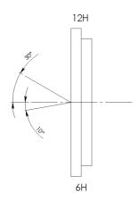
The solution is to turn the glass through 180° so you now have a 12 o'clock view which favours reading above. This also works for the other display (DMX & DDM4) products from Lascar Electronics. Unfortu-
